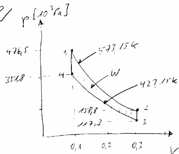
$$\textcircled{1} \quad V = 0,1 \text{ m}^3, T = 573,15 \text{ K} \\ p = 476,5 \cdot 10^3 \text{ Pa}$$
